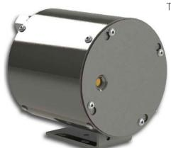
The Electron™ is Phillip Technologies's multiple crystal sensor head, designed for high vacuum thin film deposition and available in two formats. The Electron-12™ is capable of holding twelve, 14 mm industry-standard crystals, and the Electron-24™ is designed for twenty-four 8.6 mm crystals.
