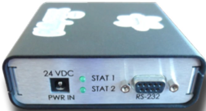
Front of the Nucleus™ showing the RS-232 port, sensor lights, and power input.
